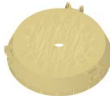
Figure 3. Strongback mesh structure for simulation with OpenFOAM
