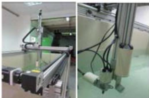
Figure 24. VISIO water facility (2 m long, 1 m large, 1 m height) devoted to ultrasonic visualisation study
