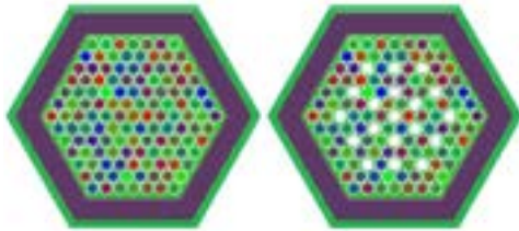
Figure 9. Control rods with small pin size (left) and control rods with moderator pins (right)
