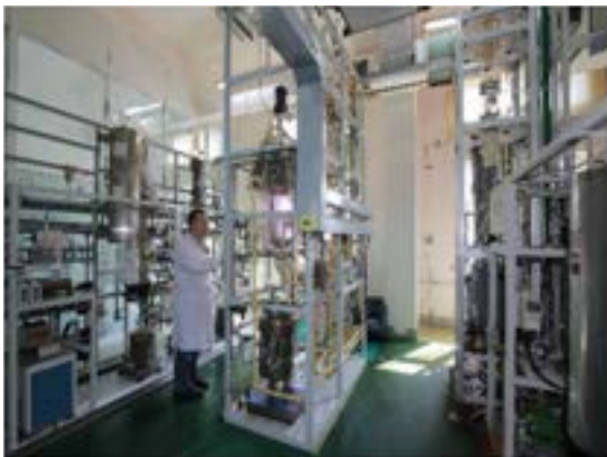
Figure 3. INET's Sulphur-Iodine process for nuclear hydrogen production
