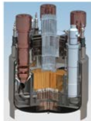
Figure 4. Integral layout of the BN-1200 primary circuit
