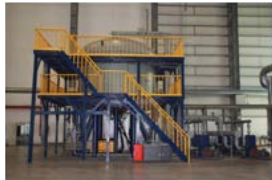
Figure 3. Pebble bed equivalent conductivity test facility
