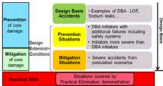
Figure 3. Illustration of design basis and residual risk
