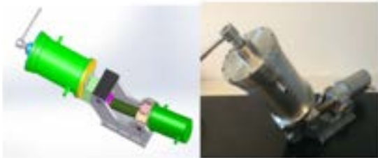
Figure 37. Specific tight robot mockup with 2 degrees of freedom
