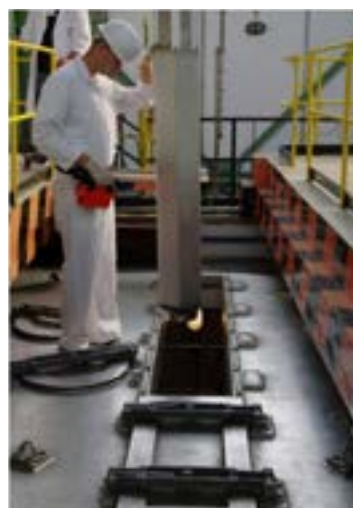
Figure 1. Loading of FLIBE zone into LR-0 reactor
