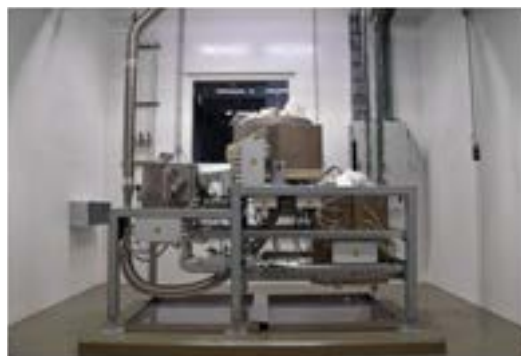
Figure 2. View of the LILLA experimental facility for mechanical testing in liquid lead
