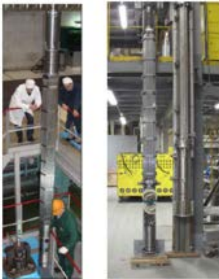
Figure 2. Full-scale FA mock-ups
