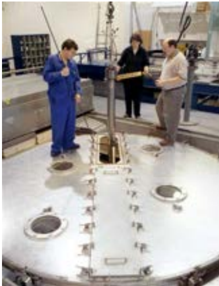
Figure 18. ZED-II Reactor for Physics Experiments in Canada
