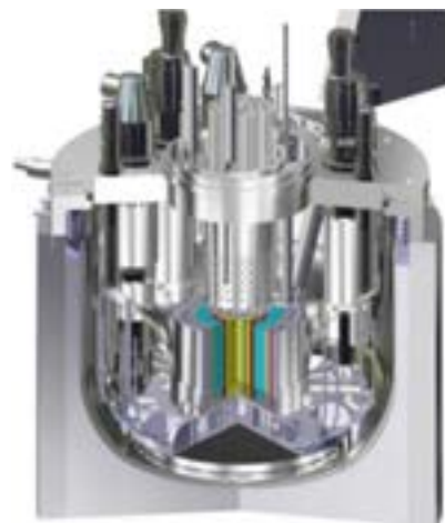
Figure 3. View of reactor vessel (© CEA-FRAMATOME)
