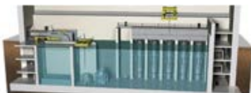
Figure 3. Illustration of the NuScale concept where the total power of the plant is spread among several (12) autonomous modules that may be add and connected as demand arises
