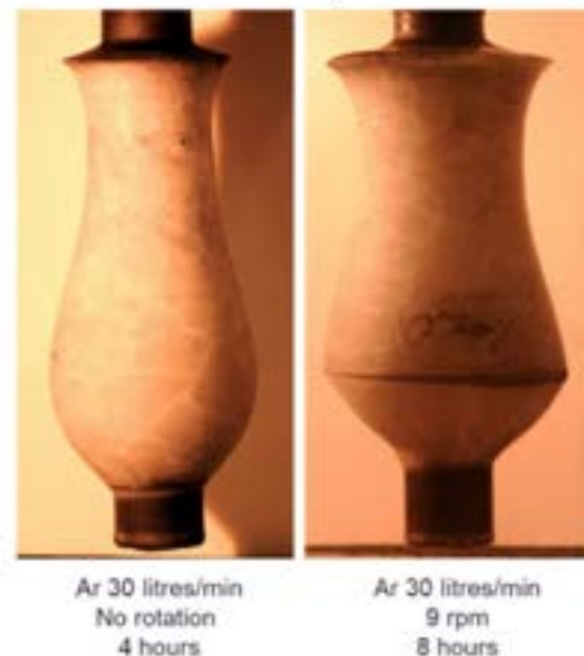
Figure 8. Flinak ingots obtained in the solidification experiments.
