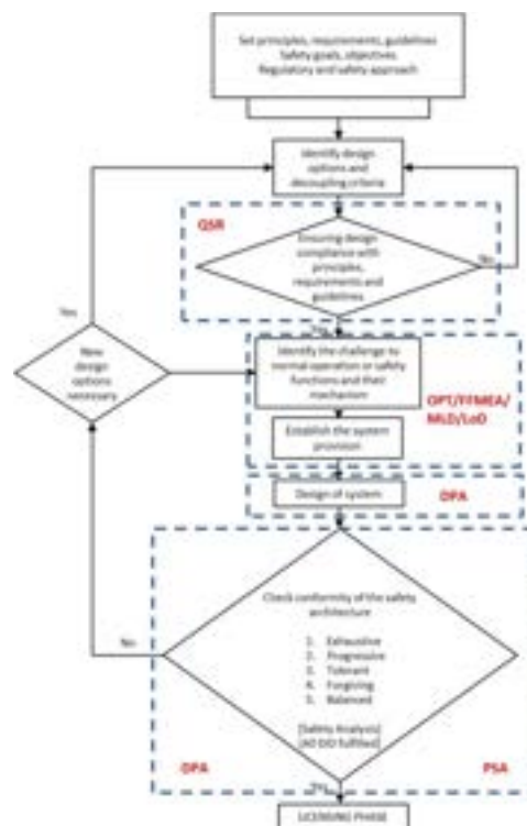
Figure 7. Flowchart of the MSFR design/safety assessment and relevance of the different tools
