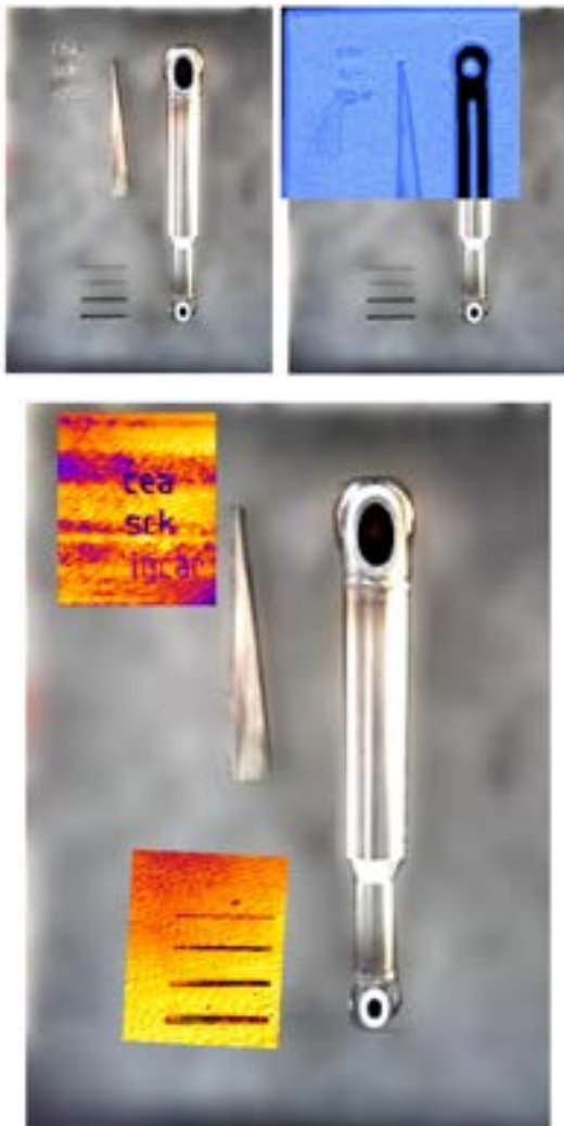
Figure 30. In sodium imaging of a plate with slits and letters (VENUS tests with TUSHT transducers). Optical image (top left), rough acoustic echoes (top right, in blue) and enhanced signal treatment (bottom, orange zones).
