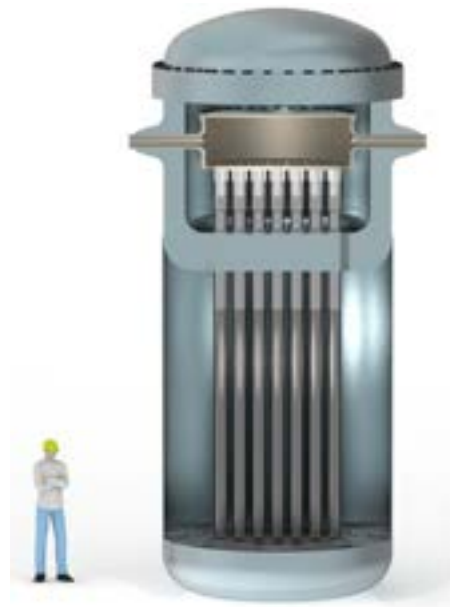
Figure 8. A Proposed Scaled-Down SCWR Core
