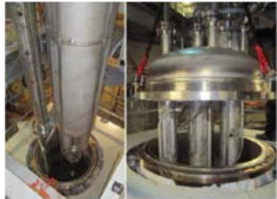
Figure 6. SGTR Test Section in CIRCE facility (MAXSIMA Project, H2020)
