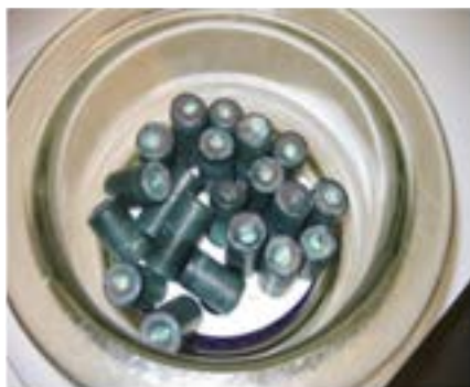
Figure 3. Frozen samples of UF 4 in FLIBE
