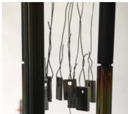
Figure 2. Coupons for general corrosion tests
