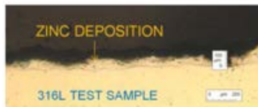
Figure 32. Metallographic cross-section – zinc deposition on 316L steel
