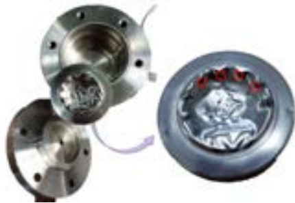
Figure 6. Result of rupture disc test
