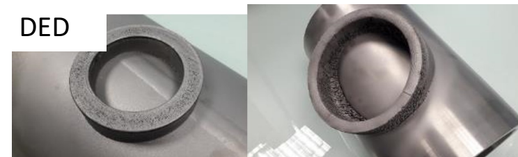
Adding a pipe connection
