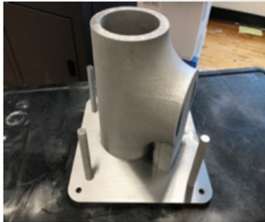
Figure 1a. A 316L SS Pipe Tee fitting is being produced via LPB-AM.
