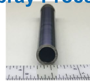
ODS coated Al-alloy mandrel Removal of Al-alloy mandrel
