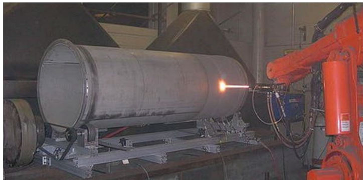
High-velocity oxy-fuel process at Caterpillar expanded to spray coat half-scale waste packages with SAM1651 amorphous metal.. https://doi.org/10.1007/s11661-009-9830-4
