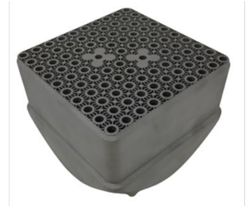
Novatech printed Lower Tie plate concept E, Inconel & SS
