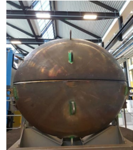
Mockup EB weld of lower head
