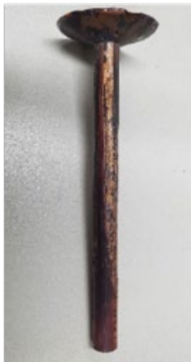
Extrusion of Cu (annular)
