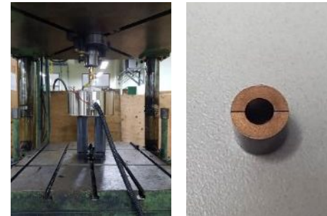
Fabrication of annular fuel(Cu)
