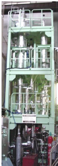
Direct-contact boiling flow loop
