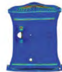
Cracking in a reinforced and prestressed concrete enclosure
