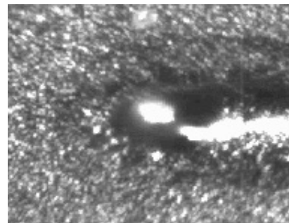
LPBF melt pool : vision with high speed camera
