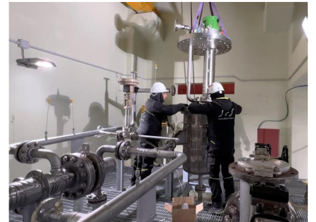
• CORE operational in March 2024 Loop-type facility to test various kinds of steel, bare and coated, in fluent lead under oxygen-controlled concentration, essentially between 10 -8 and 10 -6 wt %; temperature in the corrosion test section 650 °C and velocity 1 m/s; in the erosion test section the temperature is 520 °C and the velocity 10 m/s. It will also be used to test the effectiveness of cold traps and mechanical filters
