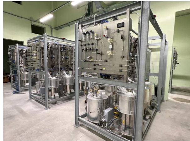
• CAPSULES operational since December 2023 Facility to test various kinds of steel, bare and coated, in stagnant lead under oxygen-controlled concentration, essentially between 10 -8 - 10 -6 wt %; temperatures span between 450 - 750 °C
