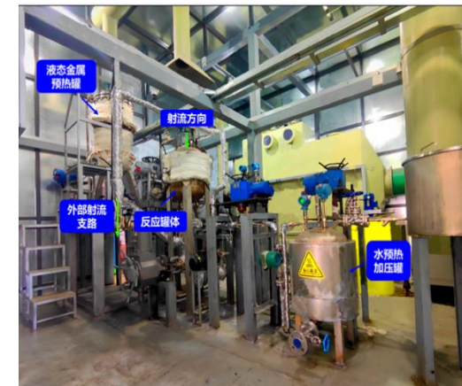
Lead-water interaction experiment by Shanghai Jiaotong Univ.
