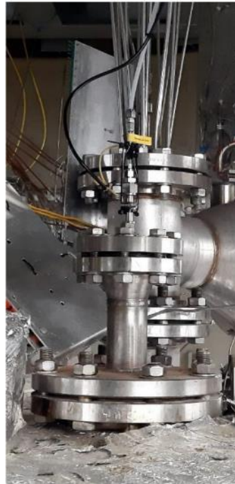
Oxygen sensors installed in the CIRCE vessel. In the hot (left) and cold (right) pool
