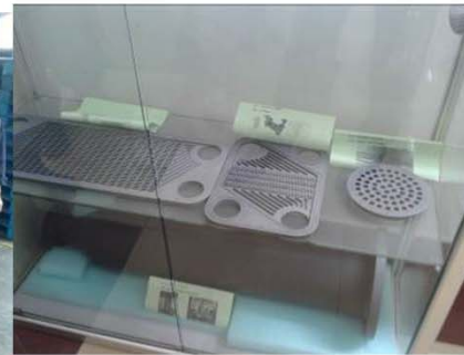
SiC heat exchanger
