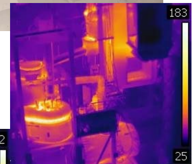
Thermal images of loop containing hot salt
