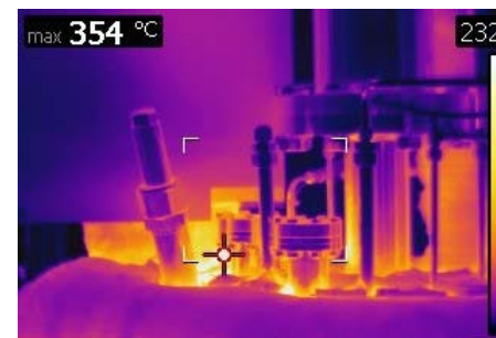
Thermal images of loop containing hot salt
