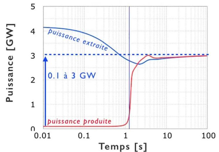
Evolution of margin to prompt criticality ( $k_p - 1$ ), of the power and of the mean fuel salt temperature for a 1 kW up to 3 GW overcooling transient with a time constant between 0 and 128s
