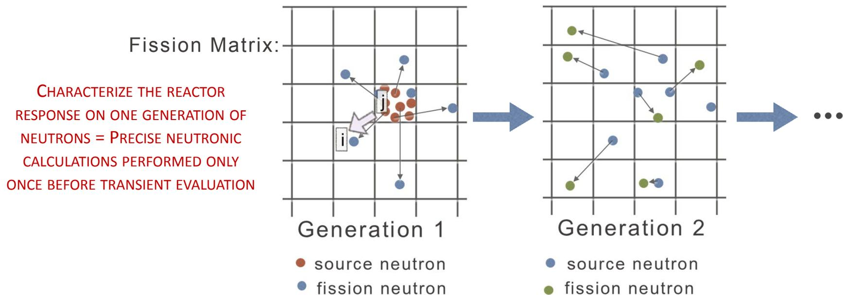
Step 1: Matrix element  $ij$  = volume  $i$  neutron production probability induced by an incoming source neutron injected in  $j$
