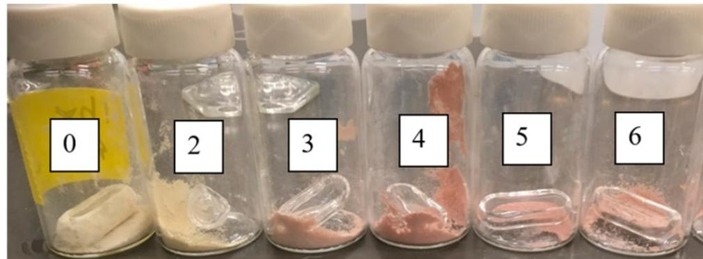
**Figure 5.** Ion-exchanged samples (45–90  $\mu\text{m}$ ) at different times of ion exchange in the increasing order of reaction time from 0 to 6 h.
