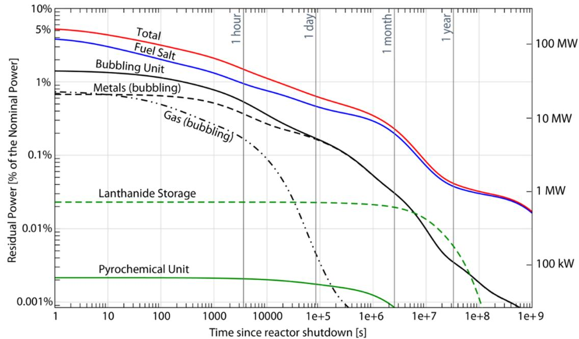
1. Reactor nominal Power: 3000MWth; 18m<sup>3</sup> molten salt.
