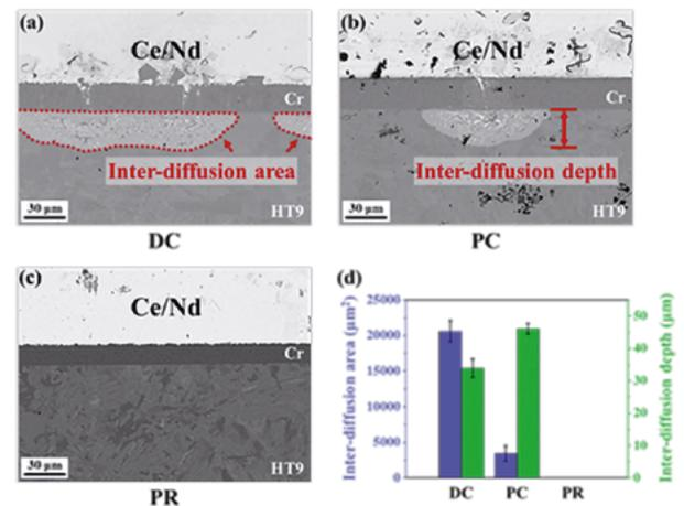
Note: (a) FCCI layer scan for direct current coating; (b) pulse current coating; (c) pulse-reverse current coating; (d) comparison of the inter-diffusion area and depths.
