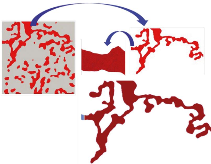
Note: Molten salt in blue penetrating into the Argon filled pores in red.
