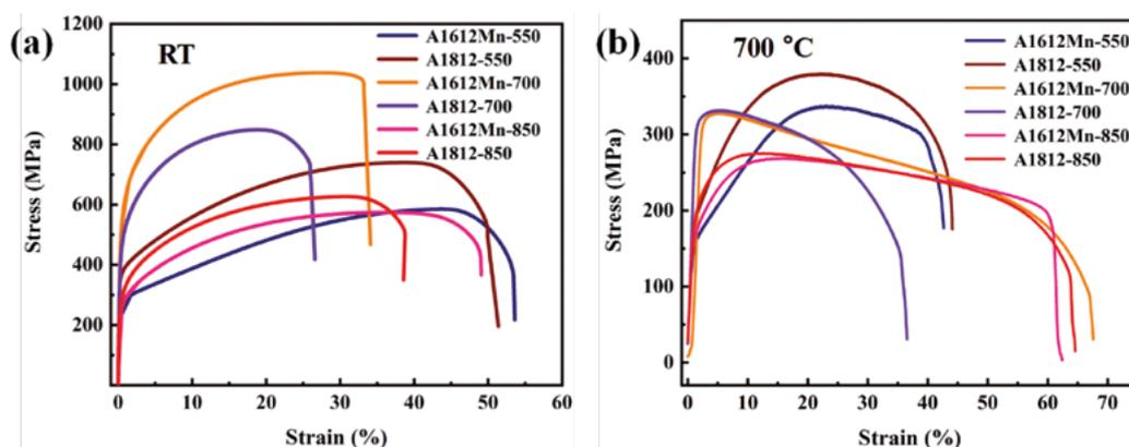
Note: The stress-strain curves of the AFA steels are shown at room temperature (a) and at 700 °C (b).
