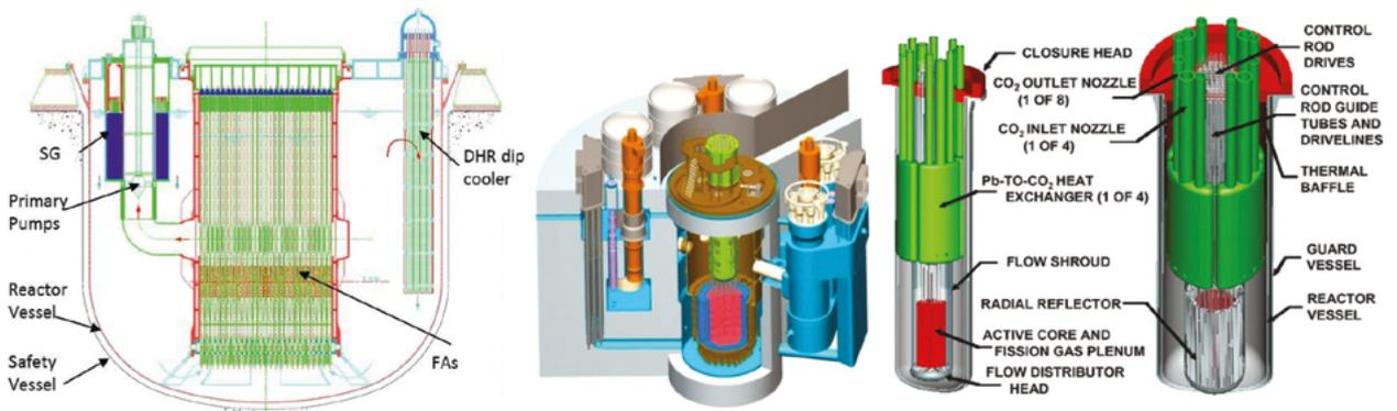
Note: The European Lead Fast Reactor (left), the BREST-OD-300 reactor (middle) and the SSTAR reactor (right).
